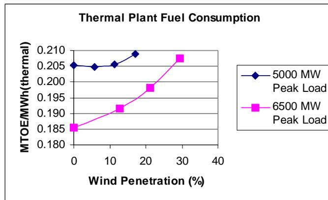
Fig 6. Thermal plant fuel consumption derived from ESB National Grid study
